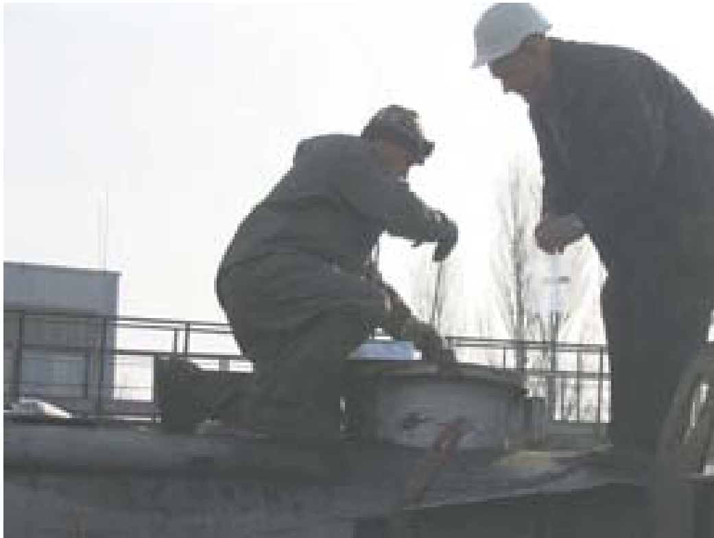
Figure 6: Sampling of the contaminated dust from the source-melting event ( ^{137}\text{Cs} ) in 2003
