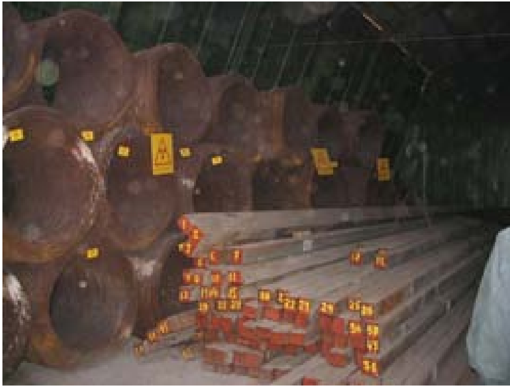
Figure 1: Contaminated steel products from the source-melting ( ^{60}\text{Co} ) event, in store
