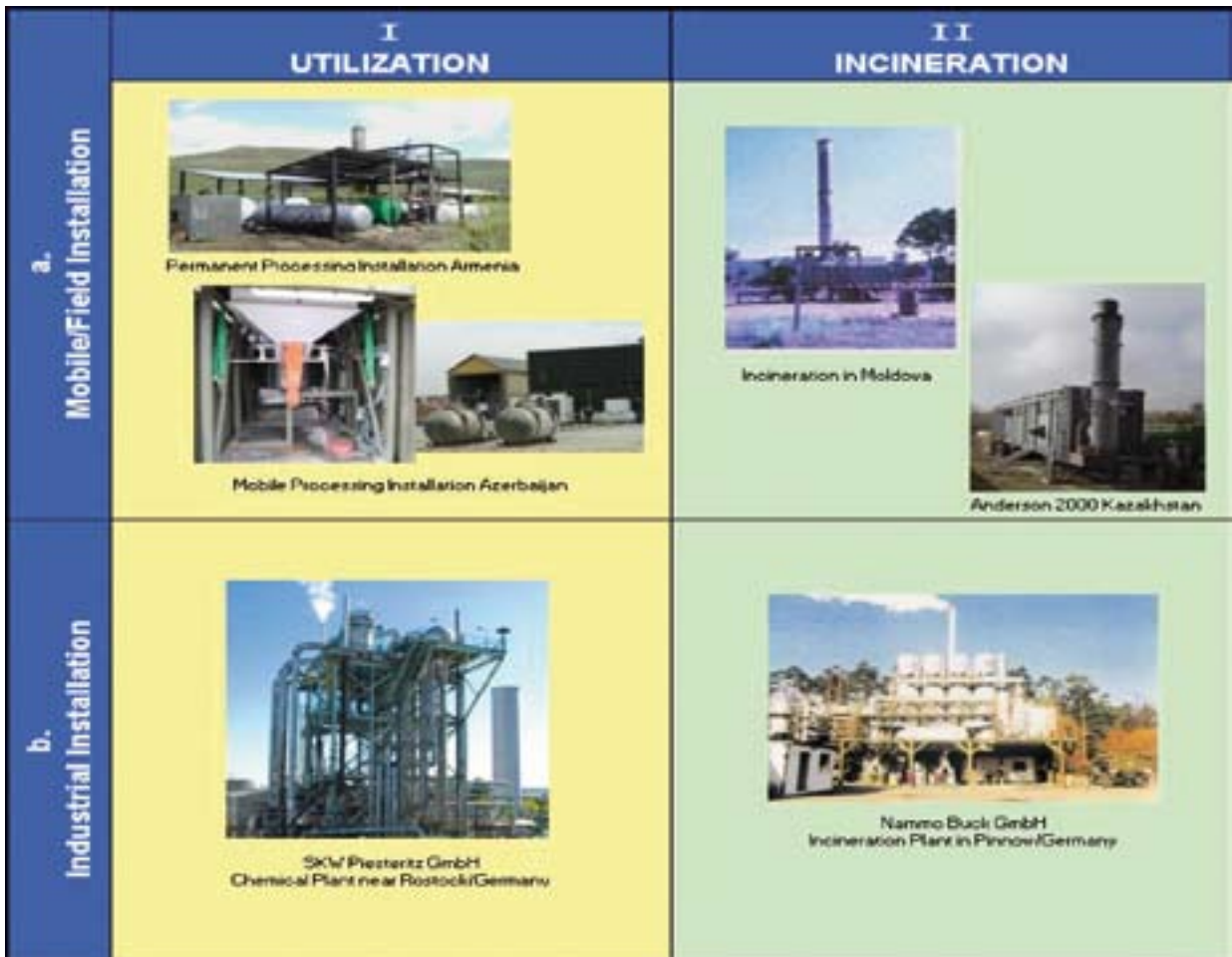
Fig. 10: Options for the elimination of melange
