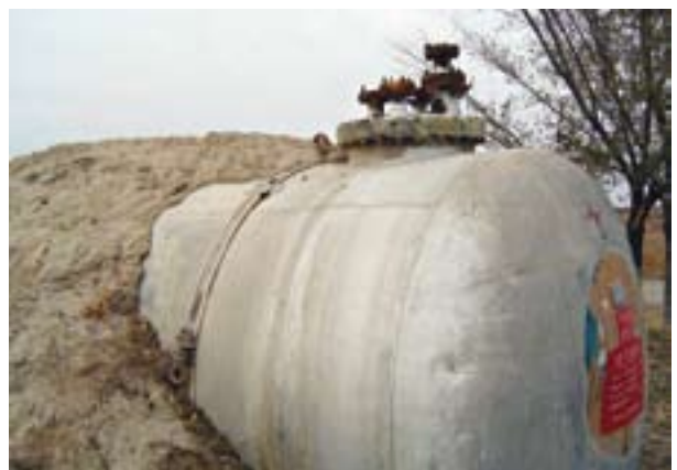
Fig. 6: Makeshift melange storage facility
