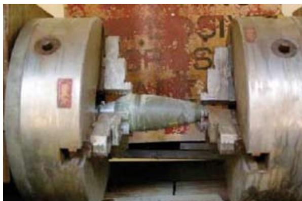
Figure 5.2: Lathe for the cutting of 81 mm mortar
