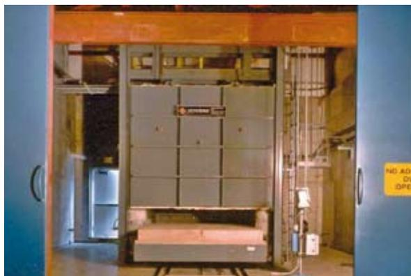
Figure 4.4: Car bottom furnace with door half open
