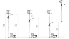
Our team has designed a unique solution to street lamps, which is supplied from wind energy and solar energy.
