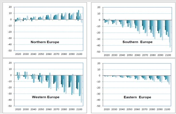
hydropower generation in TWh modelled for A1B emission scenario using different GCMs. Source: Mima, Criqui and Watkiss (2012) 10
