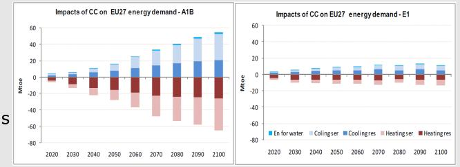
Comparison of additional cooling demand and saved heating demand for IPCC A1B and E1 emission scenarios. En for water stands for surplus energy needs for water treatment, ser stands for service sector, res for residential sector. Source: POLES model, LEPII-EDDEN, ClimateCosts after Mima, Criqui and Watkiss (2012)
