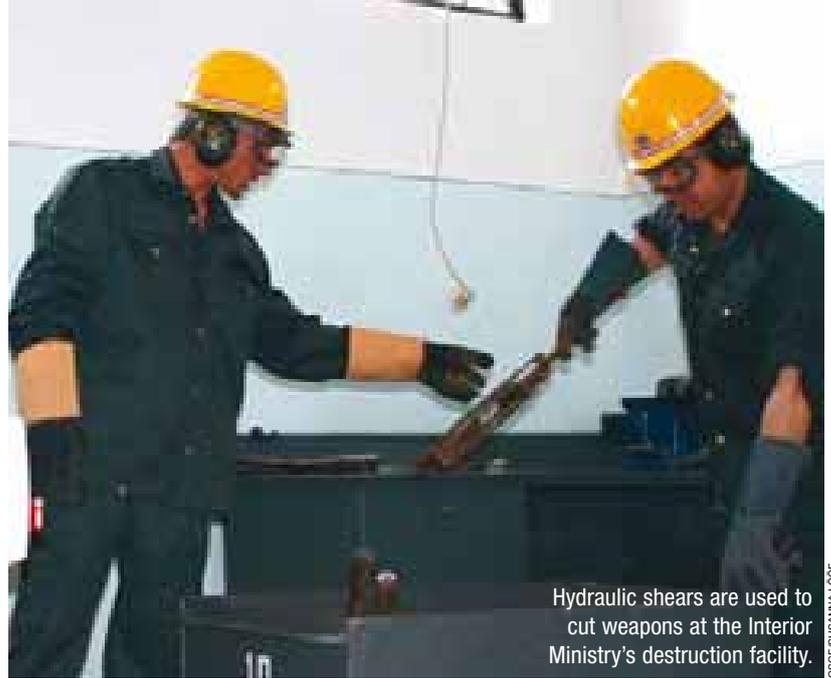
Hydraulic shears are used to cut weapons at the Interior Ministry's destruction facility.
