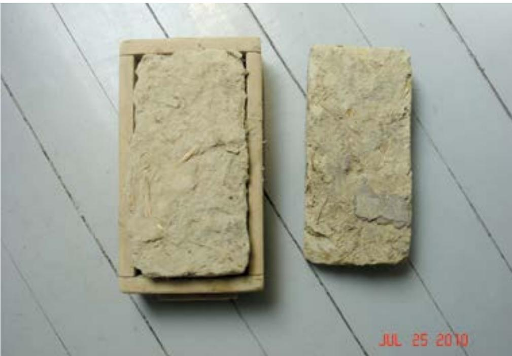
Photo 40: The mould for unbaked brick and the finished product
