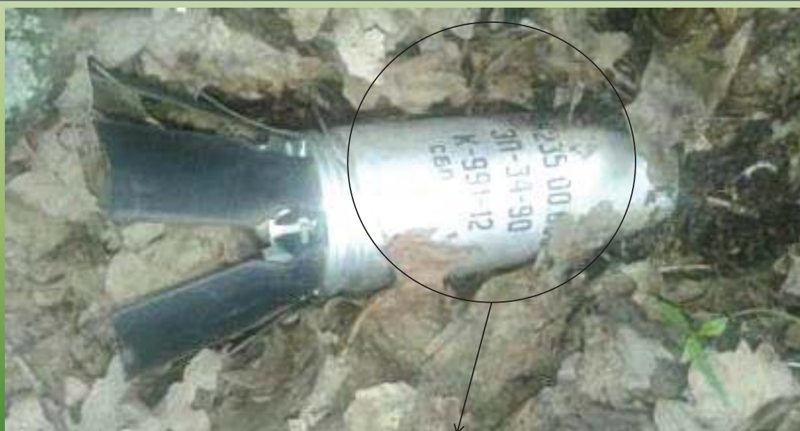
Markings 3П – rocket launcher index; 34 – serial number; 90 – year of manufacture (1990); K-991-12 – item number.
