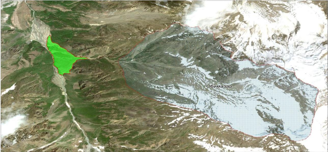
**Fig. 12. Glacial type mudflow origination site in the Obimazar river basin. The alluvial fan can cause the channel blockage and a breakthrough type mudflow (Source: Google Earth image edited by N. Ischuk).**
