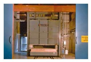
Figure 4.4: Car bottom furnace with door half open
