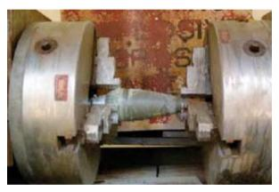
Figure 5.2: Lathe for the cutting of 81 mm mortar
