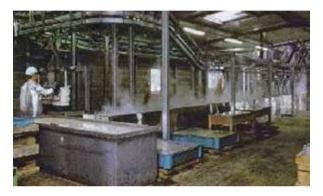
Figure 6.2: Recovery of white phosphorus using melt out
