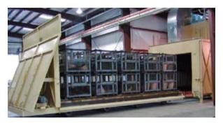
Figure 4.5: Hot gas decontamination facility. The rail car is charged with metal baskets that are loaded with pre-treated ammunition.
