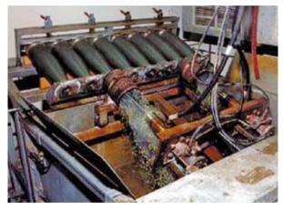
Figure 6.3: Water jet washout of 155 mm shells
