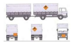
The illustration above provides examples of how to mark vehicles transporting ammunition by road by means of *warning signs*, indicating the presence of hazardous goods, and *hazard labels* (cf. Annex 6), specifically indicating that the vehicle is transporting *Class 1* items or substances like ammunition.
